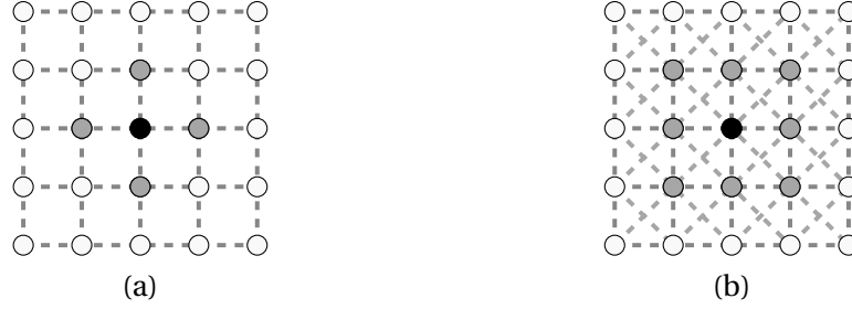
Figure 1: First and second order neighborhood graphs \mathcal{G} . (a) The four closest neighbors graph \mathcal{G}_4 . Neighbors of the vertex in black are represented by vertices in gray. (b) The eight closest neighbors graph \mathcal{G}_8 . Neighbors of the vertex in black are represented by vertices in gray.
